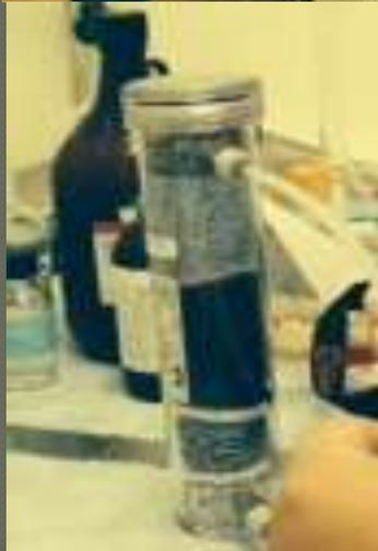
We ran the gas from the digester through two filters that we made in the lab. One filter had steel wool, activated charcoal, and Drierite™. The steel wool scrubbed out the Hydrogen Sulfide, the activated charcoal scrubbed out carbon monoxide, and the Drierite™ took out the water in the air. The Second filter we made was a water bubbler that ran the gas through deionized water to take out all the Carbon Dioxide. In the end we were left with mostly methane with trace amounts of other gasses.
